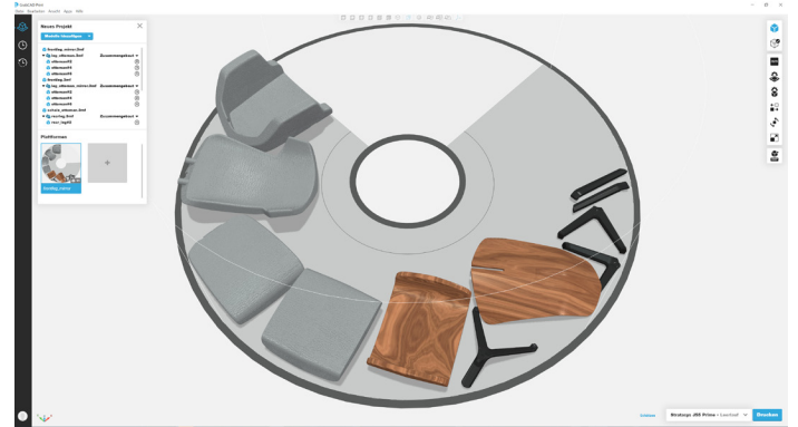
Model of a chair designed by Thinkable Studio in the GrabCAD Print Software, shown on the J55's unique rotational printing platform
