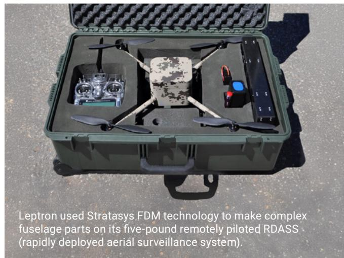
Lepton used Stratasys FDM technology to make complex fuselage parts on its five-pound remotely piloted RDASS (rapidly deployed aerial surveillance system).
