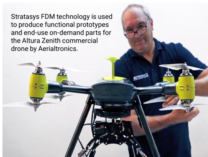
Stratasys FDM technology is used to produce functional prototypes and end-use on-demand parts for the Altura Zenith commercial drone by Aerialtronics.
