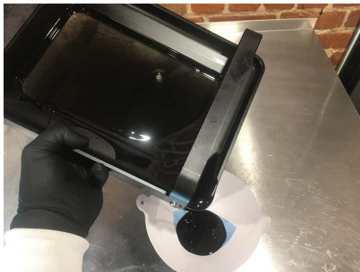
Figure 15: Empty resin tray
