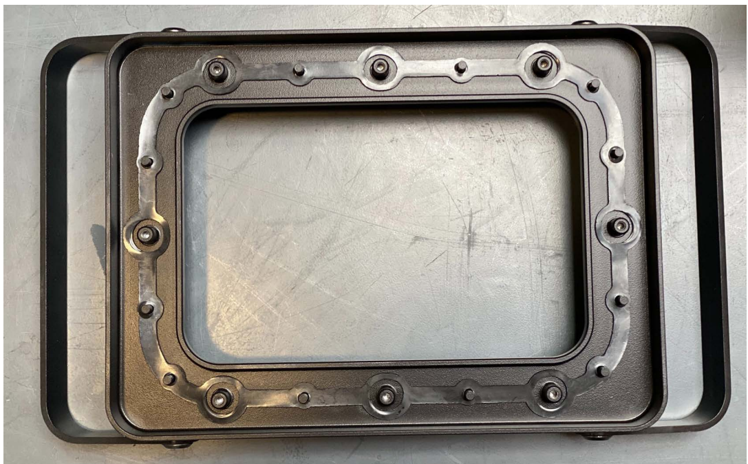
Figure 11: Gasket on tray
