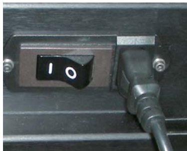
Figure 6-2: Main power switch and cable
