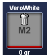
Figure 6-6: Empty cartridge indicator
