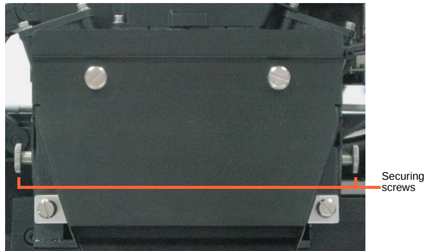
Figure 6-34: UV-lamp-assembly securing screws
