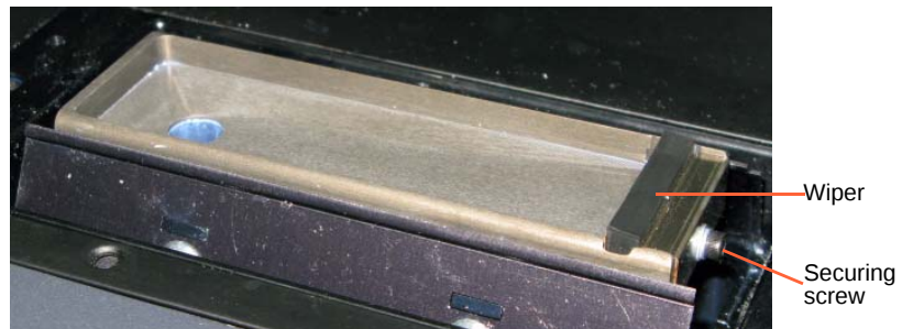
Figure 6-30: Wiper and excess-material drain
