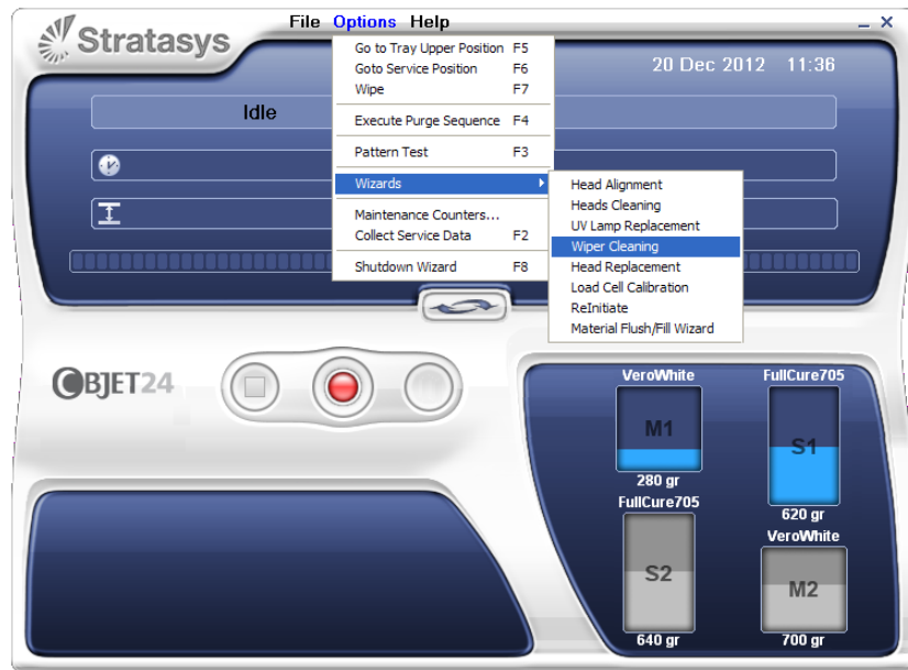
Figure 6-27: Starting the Wiper Cleaning Wizard
