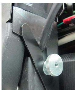
Figure 6-59: UV-lamp cable after replacing the assembly
