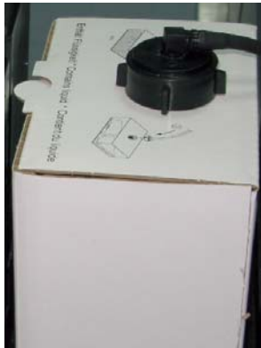
Figure 6-64: Waste container with drain tube attached
