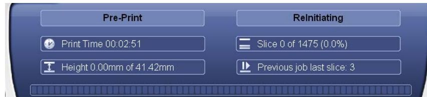
Figure 6-5: Relnitiating process during the Pre-Print cycle
