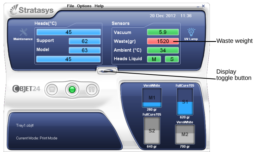
Figure 6-62: Printer interface, showing waste weight (red background indicates operator alert)
