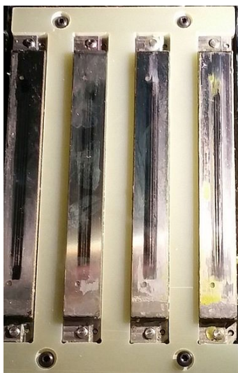
Figure 4-68 Print-head splash shield installed on the print block
