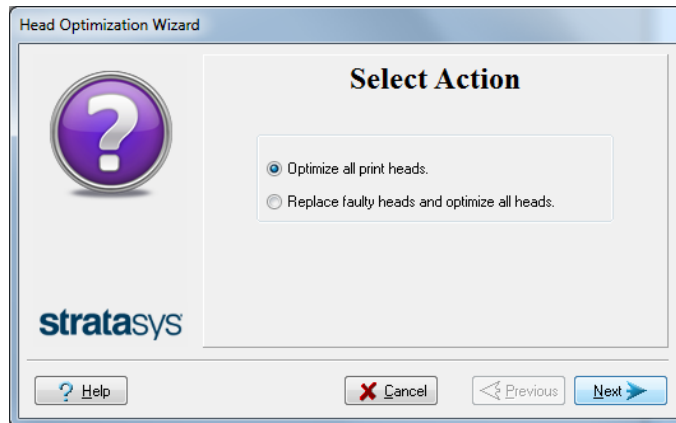
Figure 4-72 Procedure selection screen
