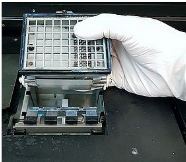
Figure 4-43 Removing the purge unit waste collector
