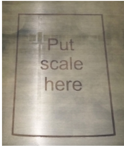
Figure 4-75 Scale positioning frame on the build tray
