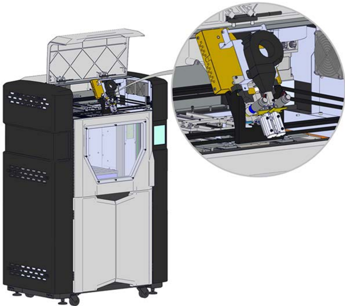
Figure 3-15: Head in Maintenance Bracket
