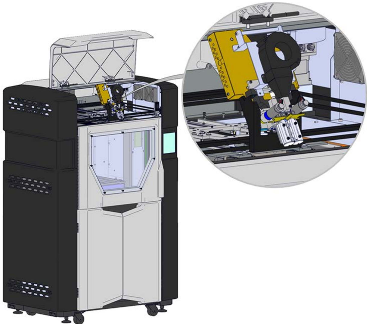
Figure 5-19: Head in Maintenance Bracket
