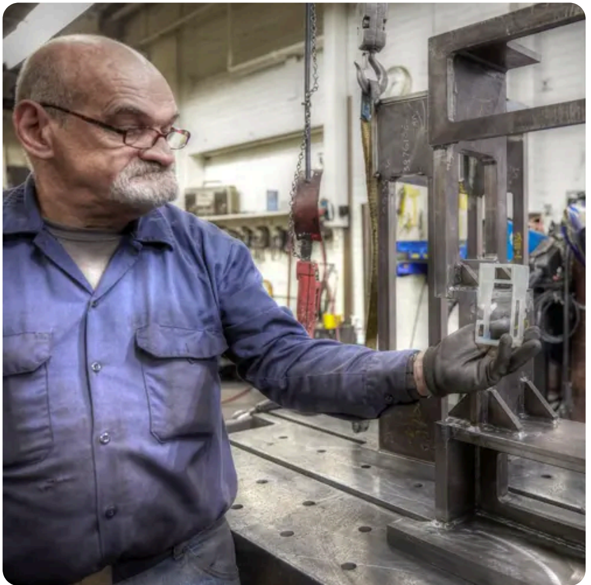
A welder at A&M Tool and Design compares a 3D printed model to the final, full-scale weldment.
